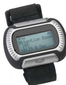
Fig.3 DECT wrist/pendant unit with text display, speakerphone, duress & dial-up communication facilities
